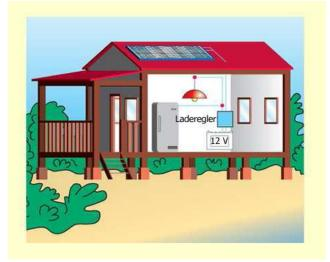
The energy needs individual, for a family house for example, (isolated site) can be covered, under the latitudes of Central Africa, by modules of a capacity from 0,5 to 1,0 kWc.
