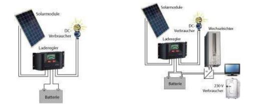
The photovoltaic systems in isolated site consist of a generator (solar panel), a different rectifier (controller of load), a storage of energy deprived (battery) and, if need be (in case of connection with electric devices, thus alternating current), a transformer of the energy (inverter). The prices for a complete system are at present in the order of 5.000 - 5.500 USD by kWc.
