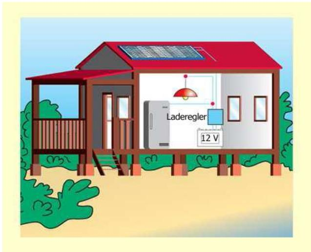
The energy needs individual, for a family house for example, ( isolated site) can be covered, under the latitudes of Central Africa, by modules of a capacity from 0,5 to 1,0 kWc.
