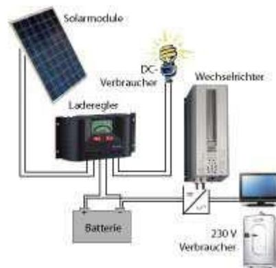
The photovoltaic systems in isolated site consist of a generator (solar panel), a different rectifier (controller of load), a storage of energy deprived (battery) and, if need be (in case of connection with electric devices, thus alternating current), a transformer of the energy (inverter). The prices for a complete system are at present in the order of 5.000 - 5.500 USD by kWc.
